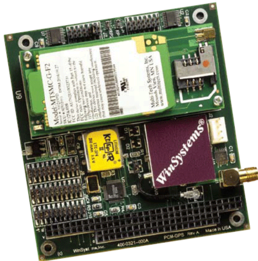
Figure 2 A representative M2M module for mobile, industrial applications, such as this WinSystems PCM-GPS, includes either a CDMA or GSM cell modem for communications and a GPS receiver for determining location.
